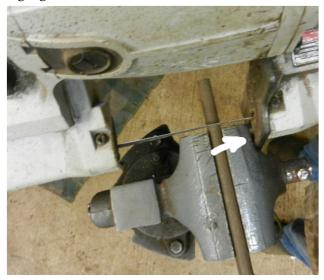
I also ground the right hand end of the jaw square so that there is a place to rest the work table of the bandsaw. The original jaw had quite an angle in this area, which led to crooked cuts or binding of the saw blade.
