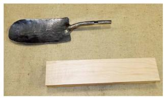
The handle is made from a piece of maple firewood that was sawn into a block,  $1-\frac{3}{4}$ " x  $1-\frac{3}{4}$ " x 10". It was then turned on a lathe. If you don't have a lathe, you can form the handle with a draw knife, spoke shave or any other carving knife.
