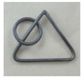
Insert one of the 6 inch rings on the triangle, forge closed and weld.
