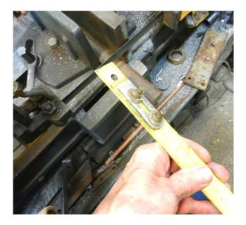
I made a dedicated measure for my bandsaw. The same idea would work for a chop saw or other metal cutting saw. I added a stop to the underside of a metal yardstick so that when I run the stop up against the casting on the frame of the saw the blade measures to the center of the blade cut.
