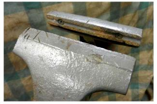
I made a couple modifications to the vise. First I ground a groove into one jaw face to better hold round bar stock. I used a grinding wheel on my angle grinder.
