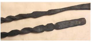
Draw out the shank to approximately  $\frac{3}{16}$ " thick being careful not to hammer the stock to thin. Hammer end to a point and form a hook. I formed the hook around a  $\frac{3}{4}$ " diameter pin. Once the hook is formed bend over the edge on the anvil. Adjust hook orientation so the flipper works well in your hand by flipping an old work glove on the anvil. Dress up the top of the eye by grinding or filing. Wire brush as needed and season using cooking oil or fat.
