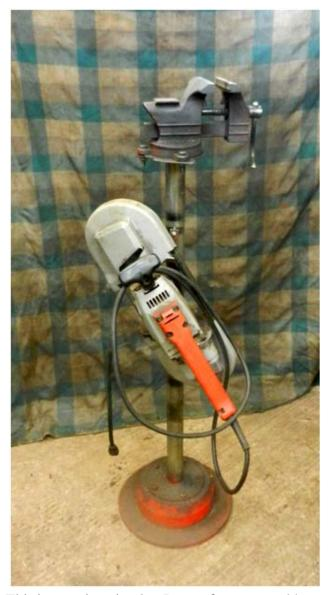
This is a cutting vise that I setup for my portable band saw. The vise is just a cheap, light duty unit that I found at the scrap yard. The stand is made from a brake rotor and some conduit. It's very light. A hook was added to hold the bandsaw. Note that the conduit is welded to a plate that is bolted to the brake rotor. Welding directly to the rotor is often not successful. I made this the same height as my big vise so that I can use them both when I need to clamp long stock.
