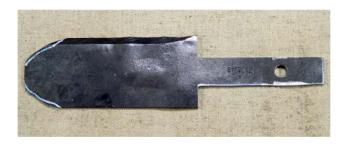
Cut away the excess material with a band saw, hack saw or angle grinder with a cutoff wheel.
