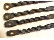
from the vise jaws sharp edges. Straighten as needed. Bring the hole to size using a ½" diameter drift, driving it through from both sizes.
