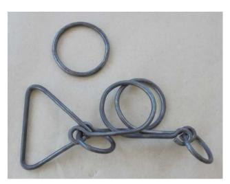
**3)** Assembly-Assemble cold by using a crescent wrench to open and close the small eyes in a vise.
