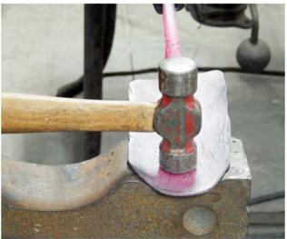
Form the blade into a curve in a swage block, table of the anvil or over the horn.
